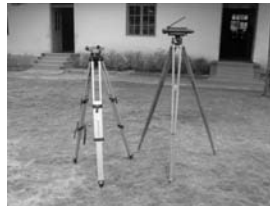
Plate 15.2 Levelling stands (adjustable and non-adjustable)
