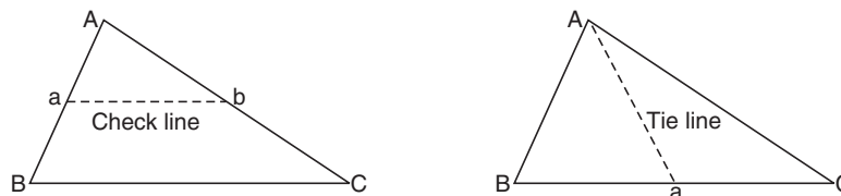
Fig. 11.4. Check line and tie line
