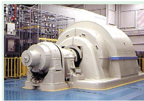
Large-capacity short-circuit current generator
