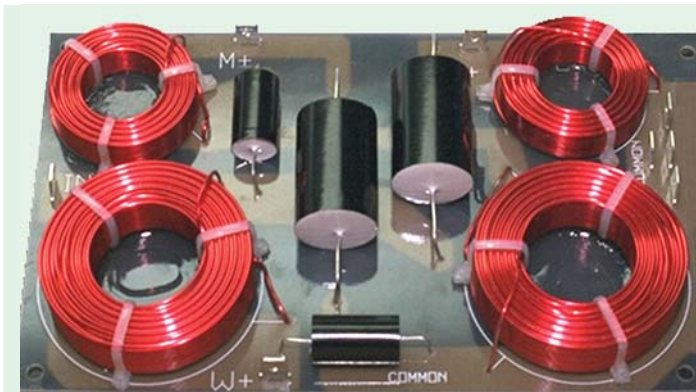
Three way passive crossover network
